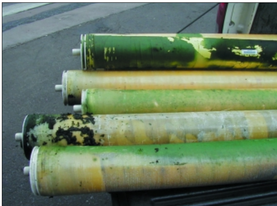
Figure 4: An example of heavy biofouling
