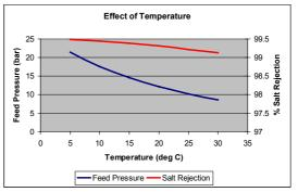
figures for temperature are 1.5-2.5% change per degree Celsius. The rate of salt passage through the membrane is also higher at increased temperatures.
