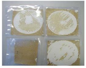
A low pH clean followed by the high pH is very effective in dealing with organic fouling. The low pH cleaner helps to break the bridge between the organics and the membrane. The high pH solution is then able to lift the foulant from the membrane surface. This is why when you clean you will sometimes only see a color change when using the high pH cleaner. Do not be misled, the low pH is a necessary and effective part of this cleaning regime.
