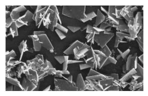
Barium Sulfate scale on a membrane, pressure vessel or pipe will feel like fine grit sandpaper. This abrasiveness can cause damage to a membrane surface during operation. When a system is started and stopped, the vexar (feedspacer) material will shift slightly. This shifting can cause the barium sulfate scale to scratch the membrane surface and cause permanent damage.
