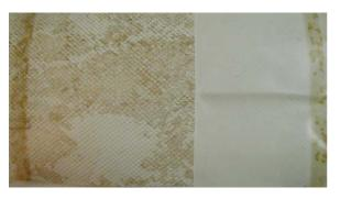
This membrane sample was taken from a single 8" x 40" membrane. The first 20" of the membrane and vexar (feedspacer) wase plugged with biological slime, the last 20" of vexar and membrane was clear. This is a good example of how biological fouling typically occurs in the front end of a system and sometimes only effects the first one or two membranes.
